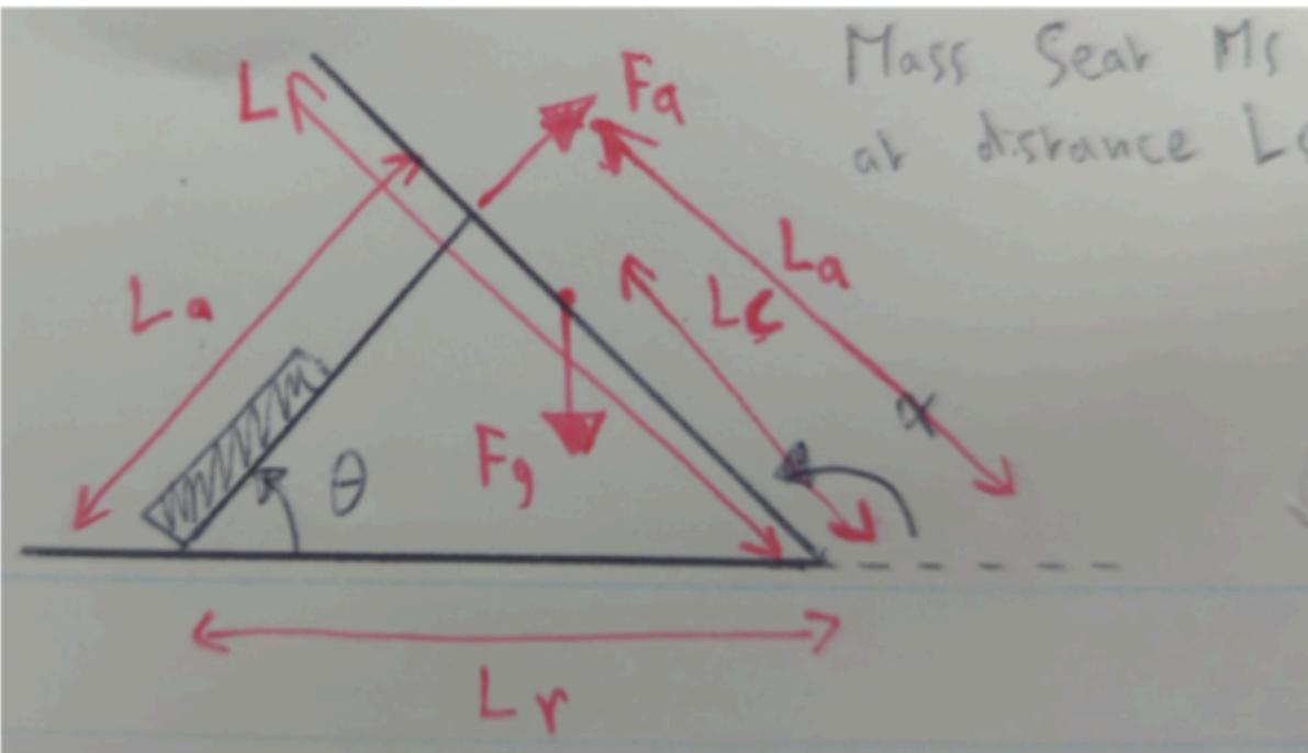
This free body diagram shows the actuator's forces as well as the person sitting on the seat.
