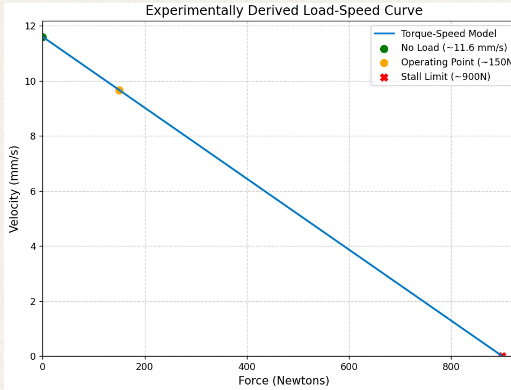
From 12V curve, we found a speed (mm/s) to PWM value ratio of approximately 0.0379 at our test load. We used this to code open-loop curve-following behavior when our sensors for our feedback variable (the seat angle) weren't working well.
