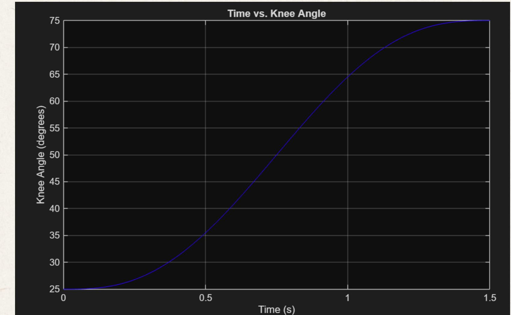
We defined a set trajectory from 25 to 75 degrees and used linear interpolation to map the knee angle  $\theta$ .
